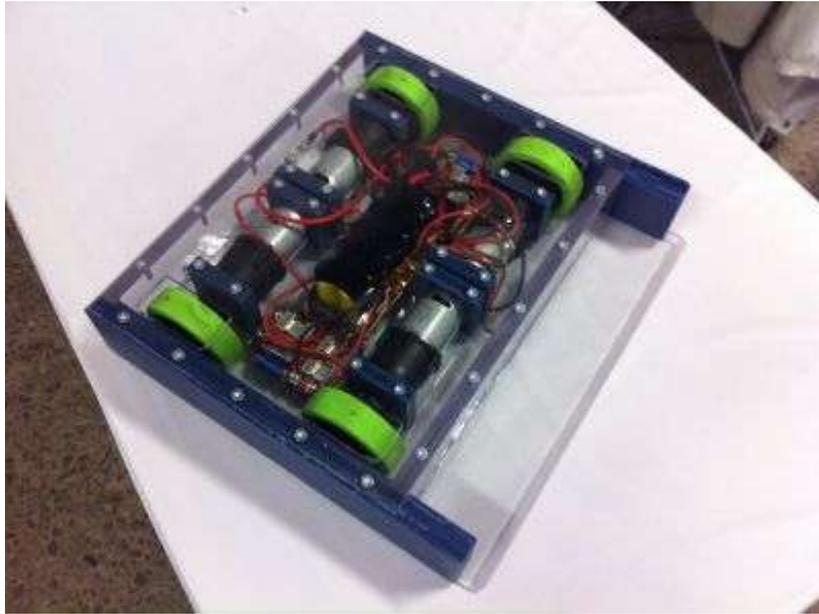
**What it is:** 12lb hobbyweight brick bot. Originally it was slated to have a front edge but (due to time) wound up with the small scoop device you can see, which we removed after it was damaged.
