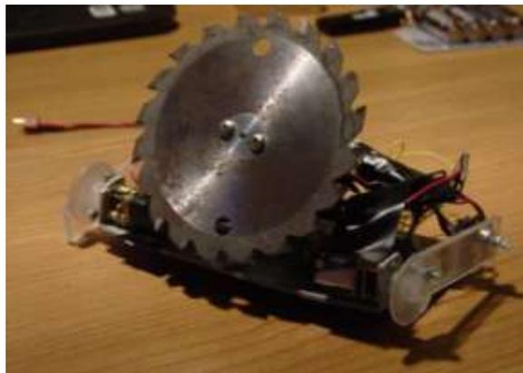
**What it was:** 150g fairyweight "shufflebot" that treaded the line between being a "walker" and being a wheeled robot. It used a simple cam system to move. It was not combat-ready but featured a sawblade weapon anyway. Its name is a play on "Robo-Sushi".
