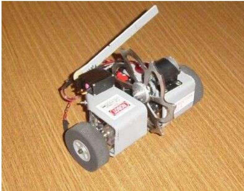
**What it was:** 1lb antweight with a vertical spinning disc. It was built out of folded ABS and polycarbonate. The original didn't have the self-righting arm that you can see at the back.
