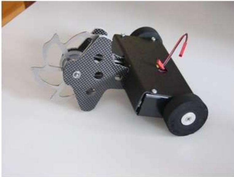
**What it was:** 1lb antweight with a vertical spinning disc. The vertical spinner had brittle (carbon fiber) weapon supports but the robot was effective.
