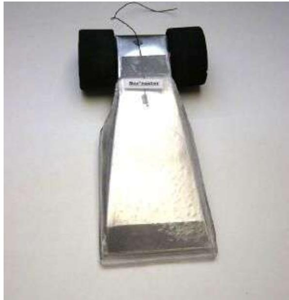
**What it was:** A 1lb antweight robot with a front flipper powered by a servo. It had a 1/32" aluminum body and the front was covered by a piece of 3/32" polycarbonate vacuum-formed to fit.
