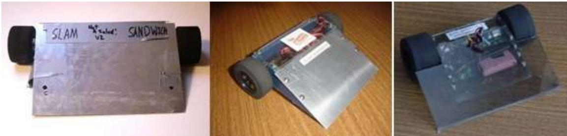
**What they were:** A long-lived series of 1lb antweight wedge robots. From left to right, Slam Sandwich (SS), Slam Sandwich III (SSIII), and Slam Sandwich V (SSV). No images of version 2 exist and version 4 was accidentally skipped!
