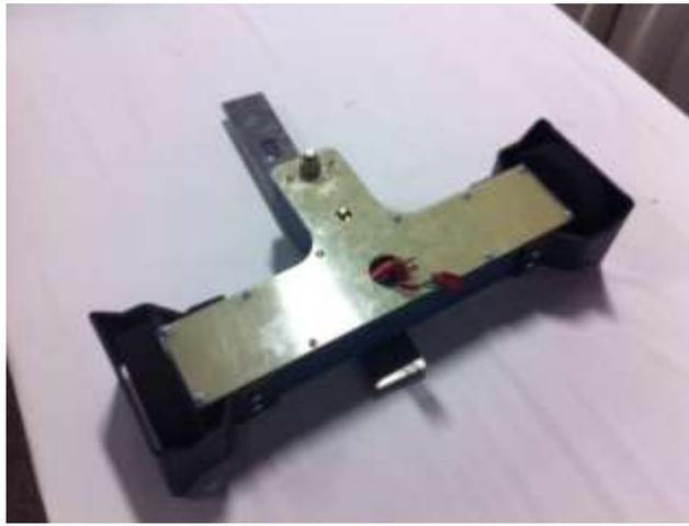
**What it is:** 3lb beetleweight robot with a (balanced) 1lb S7 steel bar.
